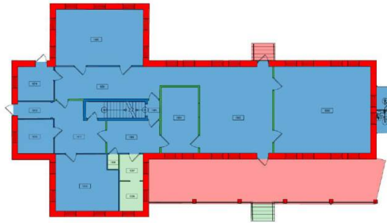
Figure 107. First floor plan showing preservation zoning. The building exterior is designated as Zone 1, including exterior stairs. The non-original stairs from the south porch are designated as Zone 3. The fire escape on the east elevation is designated as Zone 2. Most of the interior is designated as Zone 2, except for bathrooms, which are designated as Zone 3. Non-original partition walls are also designated as Zone 3.
